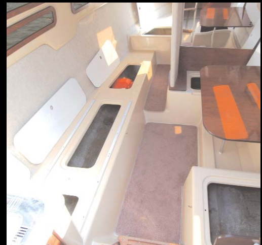
This view, looking forward, shows the storage lockers under each seat. All cushions have been removed, and the hatches opened so you can see the available space.
