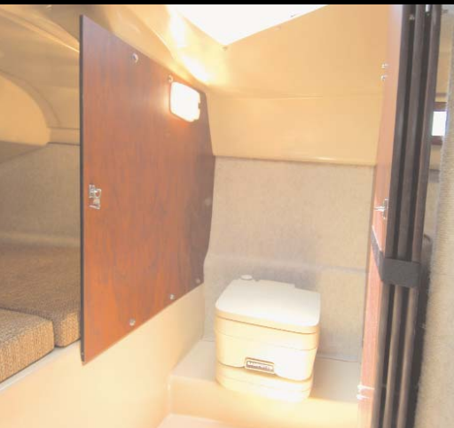
This is the enclosed head compartment. We offer a portable and removable head, but it is possible to install a conventional thru hull marine toilet and holding tank.
