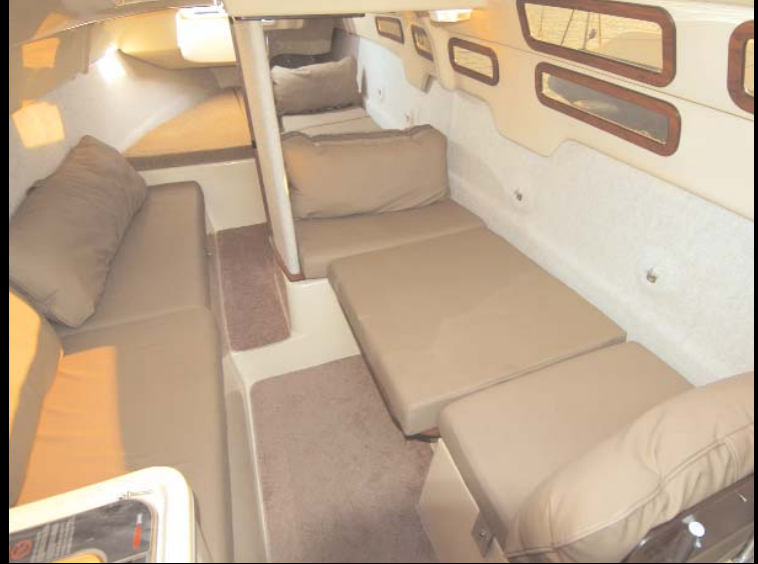
The table lowers to provide a very wide 7' 5" single berth. The 26 will sleep a total of 6 adults. This is far too large of a crowd, but it is possible. The galley is shown in the rear position, allowing for lots of seating or for a very long single berth.
