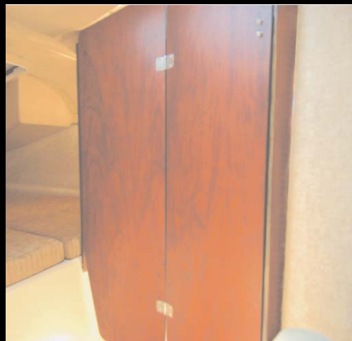
There is a good, solid head door for privacy. The door folds in the center and hinges against the back of the mirrored bulkhead. This setup is a lot better than the total lack of privacy offered by the under-bunk heads found in most small boats.
